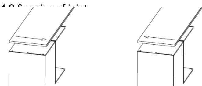
The worktop ends must be securely screwed as close to the front and back edge as possible. Furthermore, the worktop should be secured with a maximum screw distance of approx. 250 mm.
